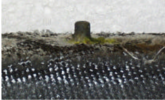
Figure 6. Recycled carbon fabric with mounting metal pin.
