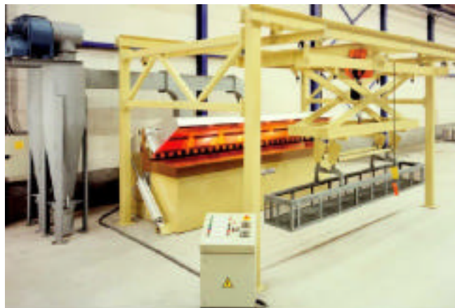
Figure 3. SEGHERS fluid Clean. The composite waste is loaded into the basket, and placed into the fluidised bed.
