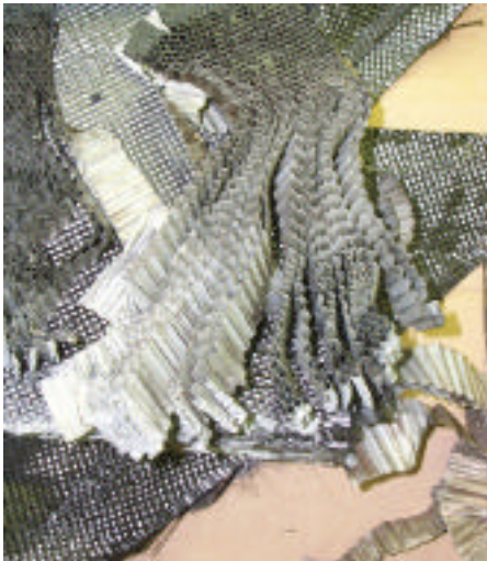
Figure 4. Recovered carbon fibres and aluminium core material.
